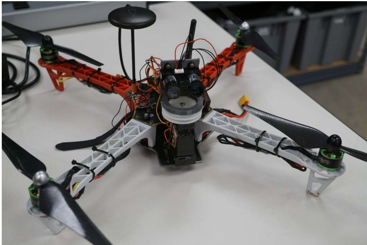
Figure 3: The updated Pixhawk-based UAS with the LiDAR light module from PulsedLight® mounted on a servo.
